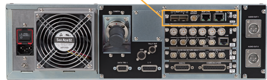
MoIP Module in exchange for the standard 12G_OUT Module
